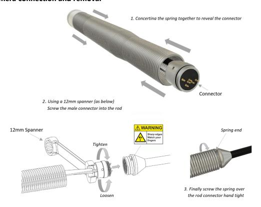
**Figure 8: Connecting the TrapJumper Camera**
